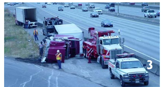
The photo sequence above shows the MIT program in action: Photo 1 shows a class S-1 tow truck preparing to move the fully loaded, rolled-over semi. Photo 2 shows the tows using cables to pull the truck from the middle of the interchange towards the side of the road. Photo 3 shows the semi fully removed from road. The interchange is once again open to traffic, and crews can begin unloading the cargo in a safer environment.
